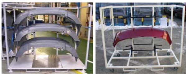
Figure 5 – Transportation units for coloured bumpers
