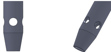
Figure 5: Nozzle modified by the insertion of 4 holes
