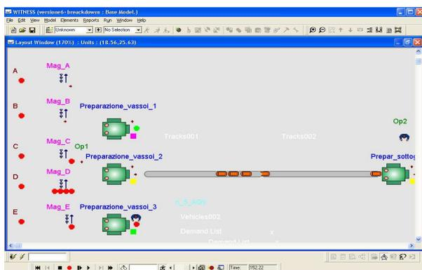
The AGV path starts from the exit of the above machines, where they load and unload the trays.
