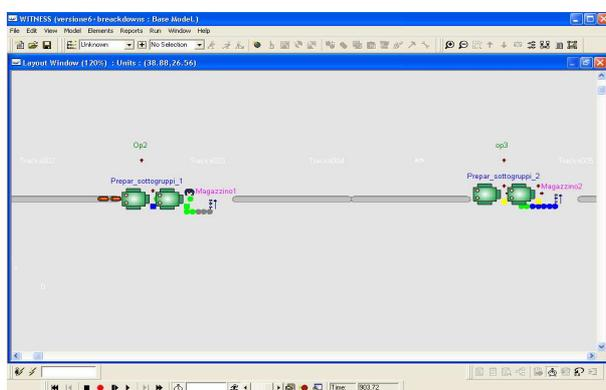
At the exit of each workstation, there is an interoperation buffer (Warehouse 1 and Warehouse 2), useful to separate the different switch production speeds. In the first buffer there are only single and
