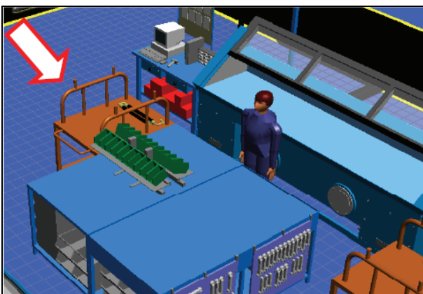
Figure 4: Manual dolly carrying the hydraulic hoses to be tested final position
