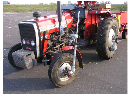
Figure 3: Testing equipment on the tractor front wheel: a) velocity sensor, b) system for measure of driven wheel position
