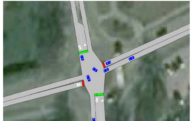
Figure 7: Scenario 3. One of roundabouts is changed to signalized intersection with protected left turns
