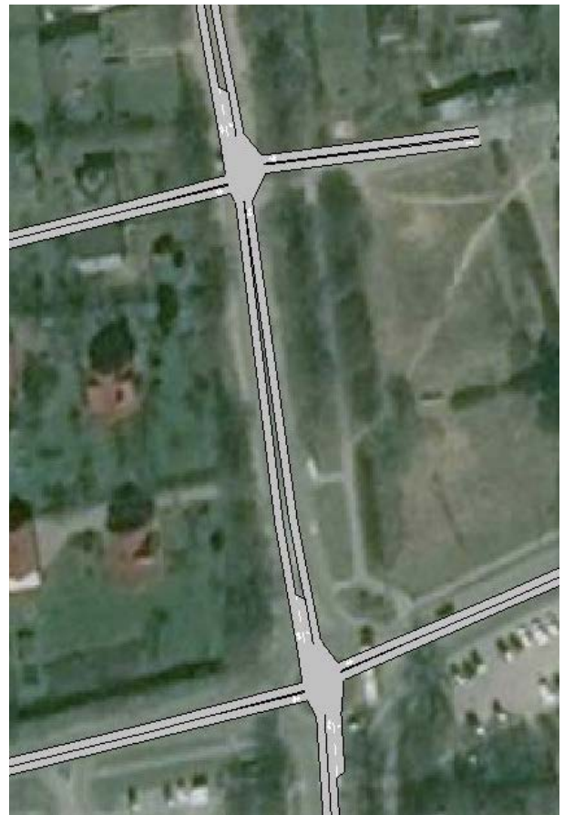
Figure 8: Scenario 4. Both roundabouts geometry is changed to signalized intersections with protected left turns
