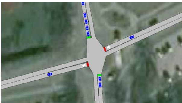
Figure 6: Scenario 2. One of roundabouts is changed to signalized intersection
