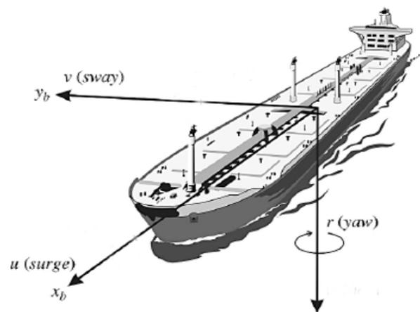
Figure 2: Movement in three DOF (Fossen 2011)
