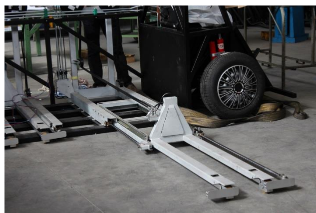
Figure 6: Robotic Handling Device: a) digital mock-up closed configuration; b) digital mock-up open and lifted configuration; c) real prototype open and lifted configuration.
