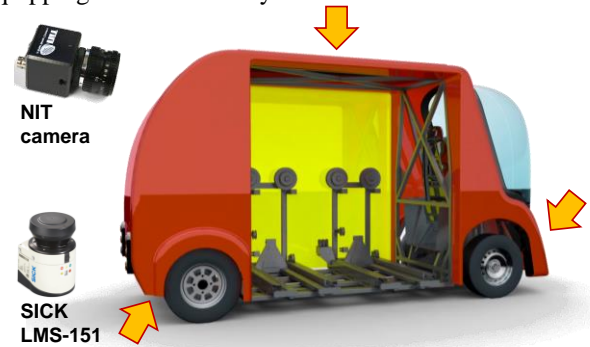
Figure 4: Main exteroceptive sensors positioning
