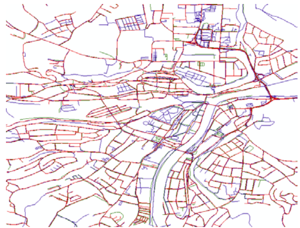
Figure 4: City of Steyr with representations of OSM (blue), GIP (green) and TomTom (red)
