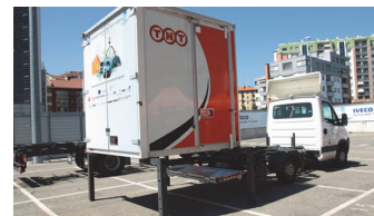
Figure 4: The Load Unit. BentoBoxes are Placed Here
