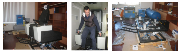
Figure. 14-16 –LamceCopeSIM40 motion platform of the ST_PT_1 simulator
