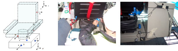
Figure 8-10 – Positioning the accelerometers on the CCIT crane operator seat for point measurements
