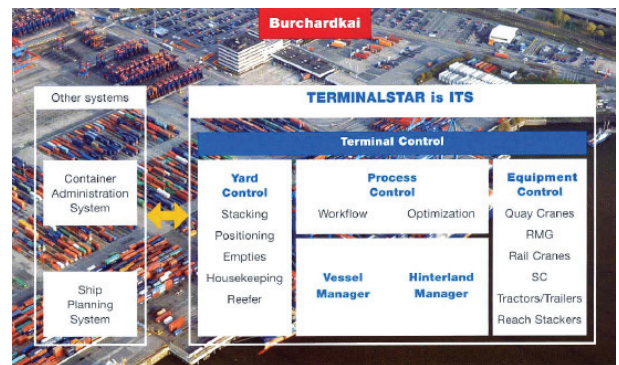
Figure 3: Softwaremodules of TERMINALSTAR implemented at the Burchardkai Hamburg
