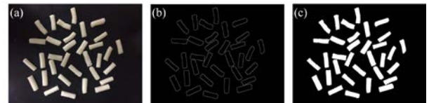
Figure 2: The overall procedure for image analysis. (a) Original image, (b) edge detected image, and (c) extracted area of the object.
