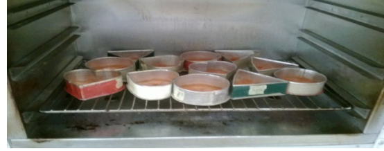
Figure 3: Sample in the Air Oven during Drying
