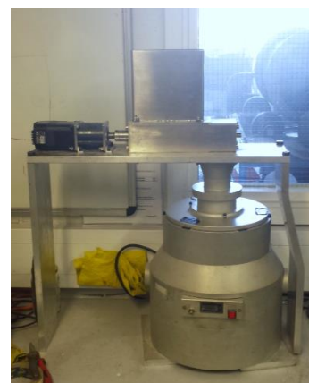
Figure 3: Centrifugal Attrition Tester
