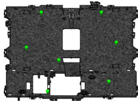
Figure 5: Injection Points on Cadmould
