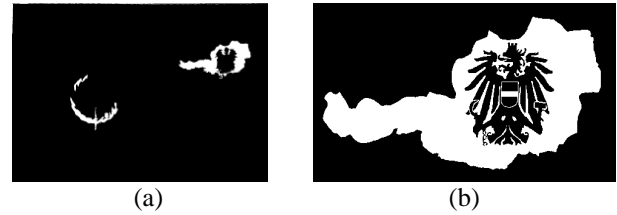
Figure 13: Hologram extracted (a) and Hologram Compare Image (b) (Austrian Passport).
