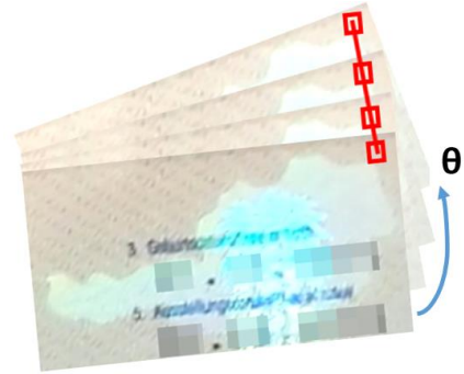
Figure 6: Line profile (red) for hologram features calculated per coordinate position for all sorted frames of varying viewing directions \theta .
