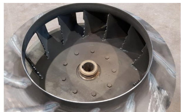
Figure 5: Manually Pre-Damaged Impeller.
