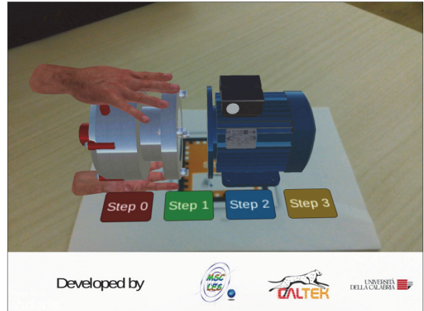
Figure 13: Detach/Attach the main pump body
