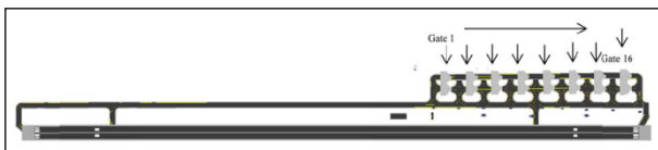
Figure 7: Configuration taxi-in taxi-out concept
