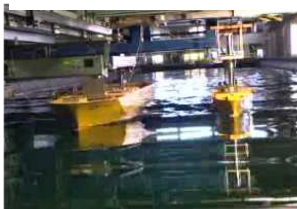
Figure 10 – Tank test for interaction forces
