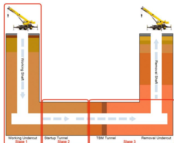
Figure 1: Trenchless TBM Tunnel Components and Initial stages of Tunnel Excavation
