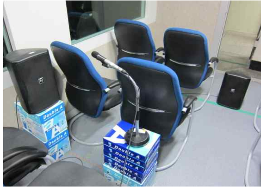
Figure 15: The ANC system in the test-bed at the 110cm height
