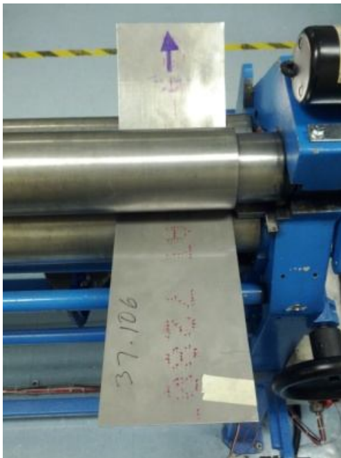
Figure 5: Roll bending process experiment
