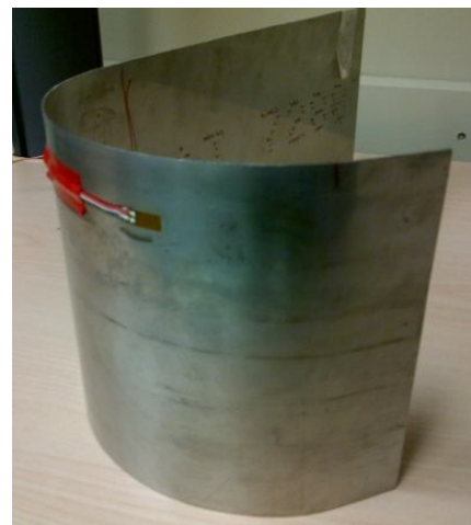
Figure 11: Workpiece after roll bending process
