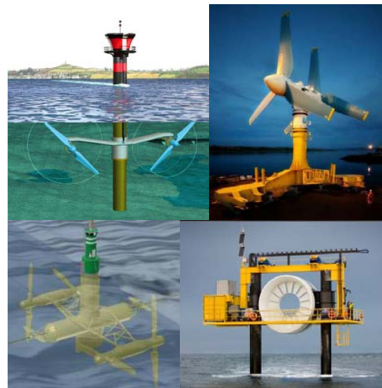
Figure 1: Sea-Gen, Atlantis, Morild & Open-Hydro TECs
