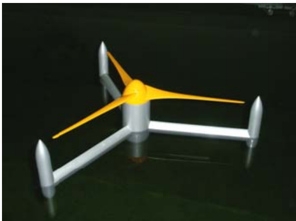
Figure 5. Scale Model of GESMEY Device in Maintenance State.
