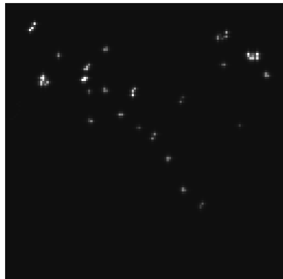
Figure 5: images from a surface inspection application with flaws concentrated in the upper half of the image except a line-like structure from the upper left to the lower left.
