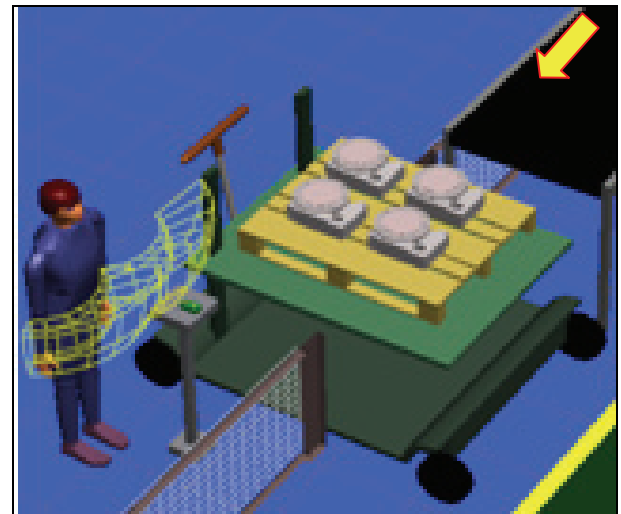
Figure 13: Final workstation configuration for the carrying the assembled work piece to the mechanical arm location
