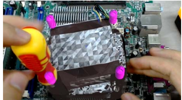
Figure 10: Remove the pink rendering screws.
