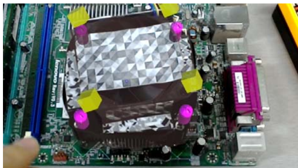
Figure 9: Open the project scene, air tap to start the maintenance process..
