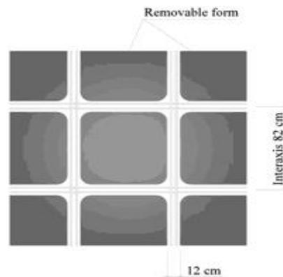
Figure 3 features of the selected slab
