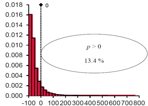
Figure 3. *Fr 13* simulation of *on-only* energy cooling strategy with 5,000 scenarios. The 670 failure scenarios (13.4 %) are shown to the right of the figure ( $p > 0$ )
