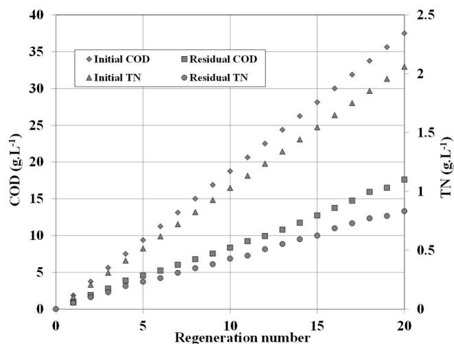
Figure 4: Initial and residual COD and TN of NaOH solutions over successive regeneration cycles.
