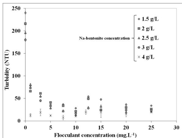
Figure 3: Effect of reactant concentrations on turbidity in NaOH regenerated solutions
