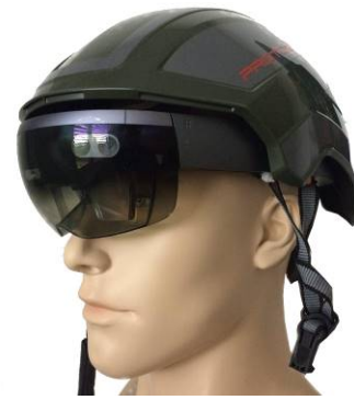
Figure 8: Microsoft HoloLens in Helmet.
