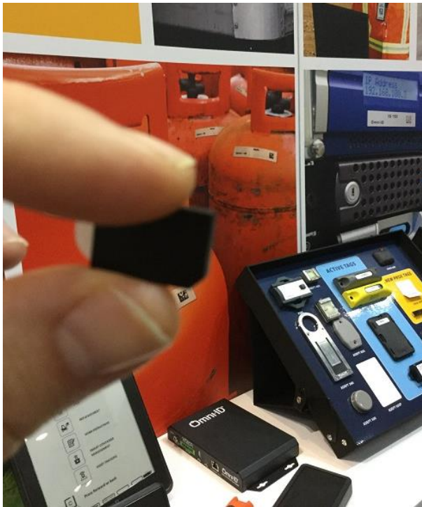
Figure 1: On Metal RFID Tag for Drill-pipes (taken at RFID Journal Live 2018)
