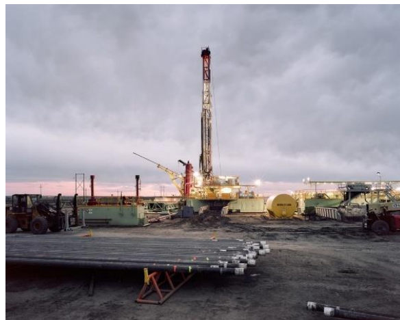
Figure 5: Drill-Pipes on a Rig
