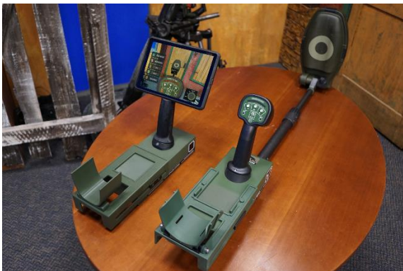
Figure 2: Low-Cost Surrogate (Left) Real Device (Right)
