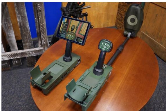
Figure 2: Low-Cost Surrogate (Left) Real Device (Right)
