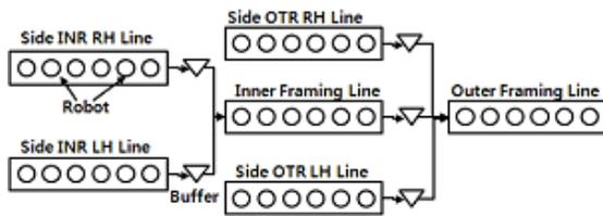
Figure 3: Abstract Layout of Layered Build Method (Wang, 2014; Kim et al., 2015; Moon et al. 2016)
