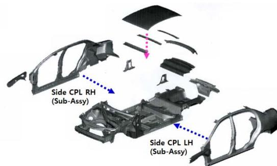
Figure 2: Concept of Modular Build Method (Kim et al. 2015; Moon et al. 2016)
