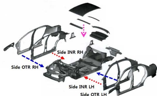
Figure 1: Concept of Layered Build Method (Kim et al. 2015; Moon et al. 2016)
