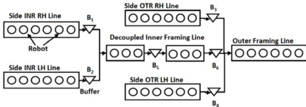
Figure 5: Decoupling Sub-line in Layered Build Layout
