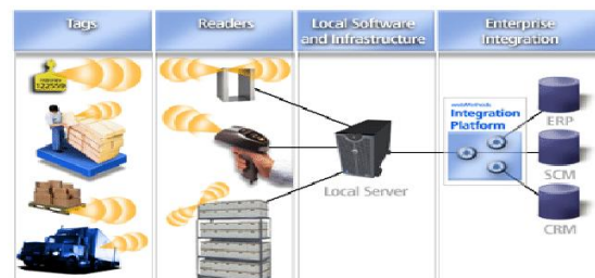
Figure 02 - Basic scheme of RFID use.
