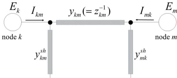
Figure 1: A diagram of node  $k$ , node  $m$ , and a transmission lines between these nodes.
