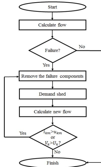
Figure 4: A flow chart of cascading procedure considering demand shedding
