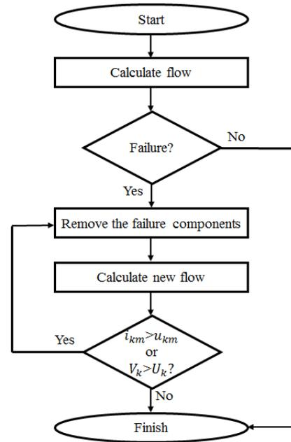
Figure 2: A flow chart for cascading procedure
