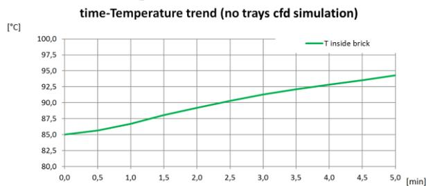
Figure 13 Time-Temperature trend in the local point inside the brick
