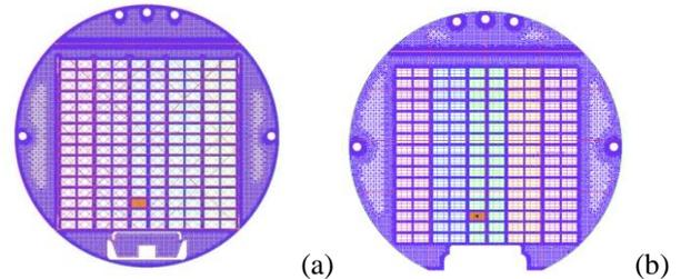
Figure 5: volume mesh of the configuration with trays (a) and without trays (b)
