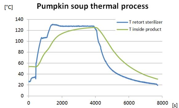
Figure 14: Temperature trend of the retort room and inside the brick
