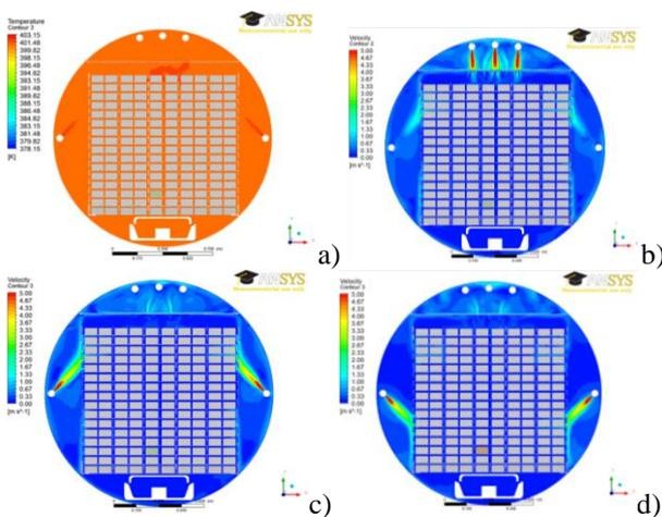
Figure 9: Temperature inside the sterilizer a); velocity inside the sterilizer at 3 planes: b) c) and d)
