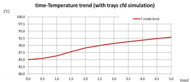
Figure 11 Time-Temperature trend in the previously defined point inside the brick
