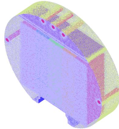
Figure 4. External mesh surface
