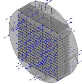
Figure 6. Boundary condition in CFX-Pre Solver
