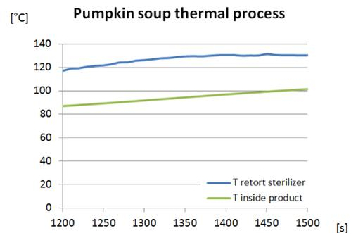
Figure 15 Temperature trend of the retort room and inside the brick in the reference time (1200-1500s)
