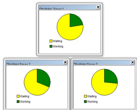
Figure 9: Utilization of shaping machine EMAG
