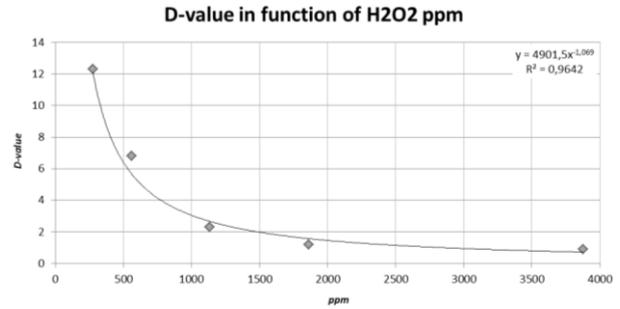
Graph 1. D-value in function of H<sub>2</sub>O<sub>2</sub> ppm for the Weibull model
