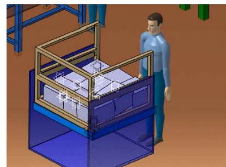
Figure 12. Proposed Workstation to Reduce the Ergonomic Risk of the Placement Operation.
