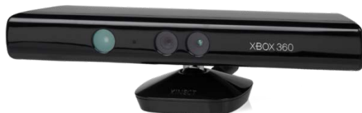
Figure 1. Depth Sensing Device. (Source. Wikipedia Commons file “The Microsoft Kinect Peripheral for the Xbox 360”)
