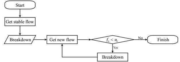
Figure 1: A flow chart for cascading failure
