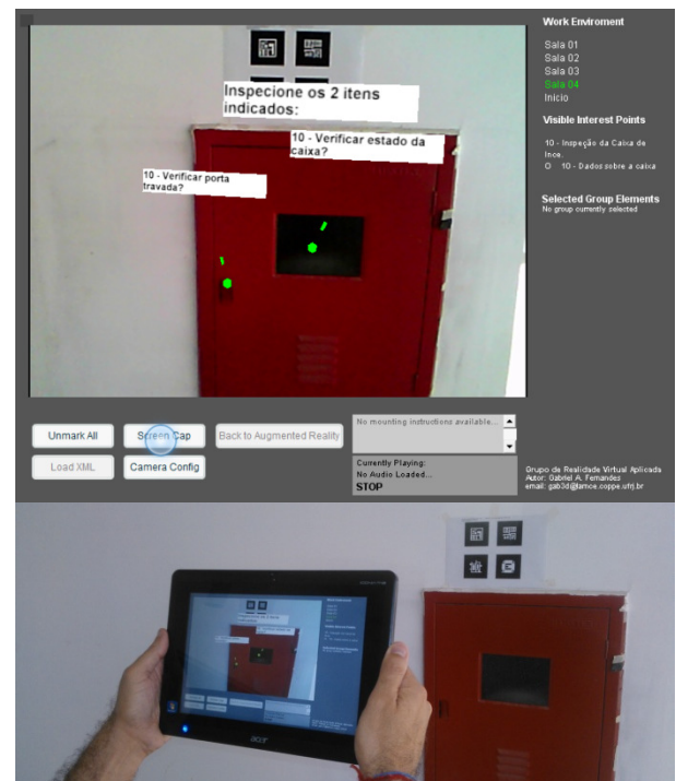
Figure 3. Fire hose box; top: application screenshot; bottom: user holding the tablet.
