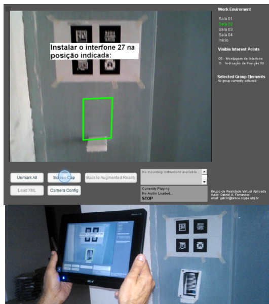
Figure 5. Top: Assembly task screenshot; Bottom: user inspecting installed part in place.
