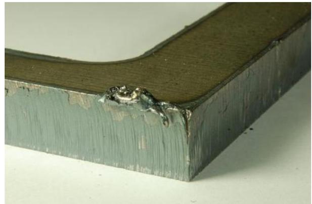
Figure 1: Periodic Striations and Adherent Material at the Cut Edges, 8mm Steel
