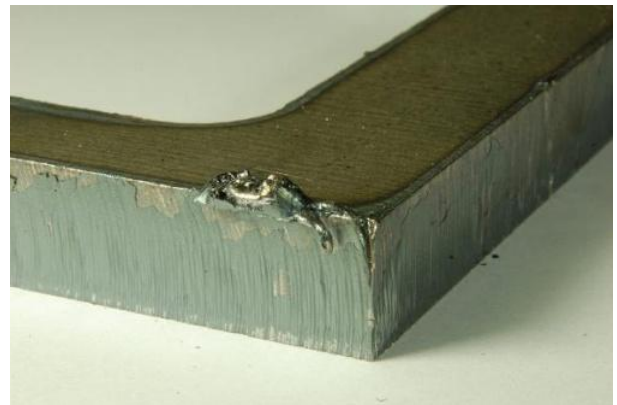
Figure 1: Periodic Striations and Adherent Material at the Cut Edges, 8mm Steel
