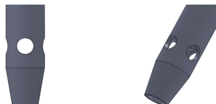
Figure 5: Nozzle modified by the insertion of 4 holes
