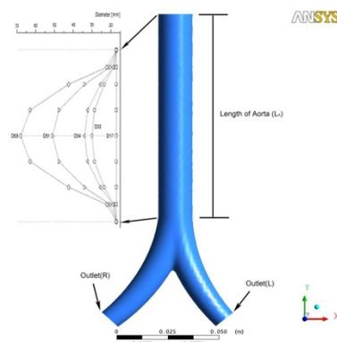
Figure 3: Diameter of each models
