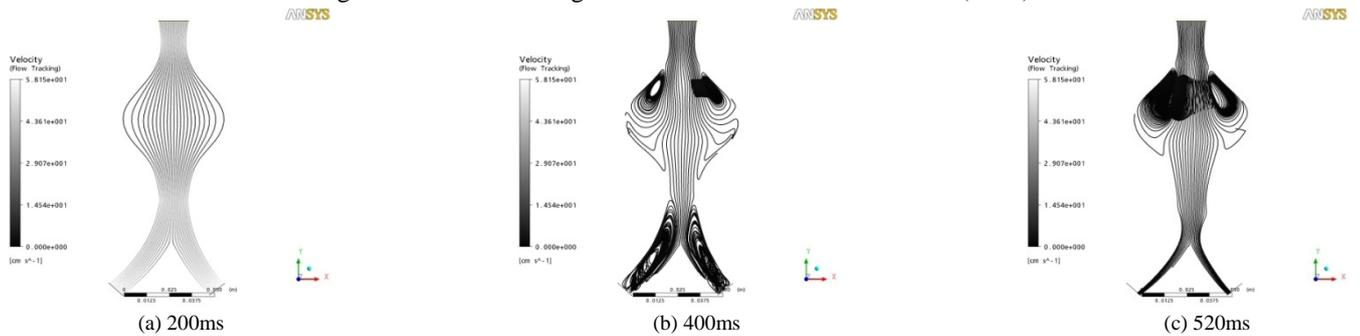
Figure 10: Flow Tracking Line of Normal Abdominal Aorta (D:64)
