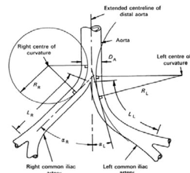
Figure 2: Standard model of abdominal aortic aneurysm
