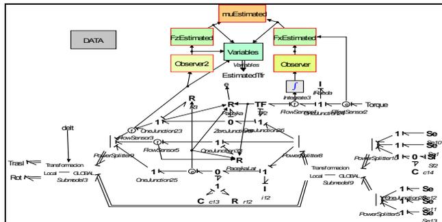
Figure 8: Suspension System with Observer and Estimate modules
