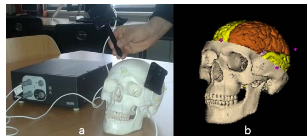
Figure 5: Phantom with attached position tool, surgical pointer and tracking unit (a), and segmented image space (b).
