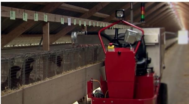
Figure 7: Robotic mink feeding system based on Norcar Minkomatic vehicle.
