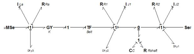
Fig. 3. Simplified BG model of the torsion bar
