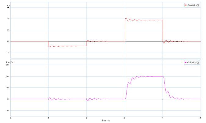
Fig. 6. Output variable  $y_1(t)$  and control  $u(t)$  with disturbance rejection
