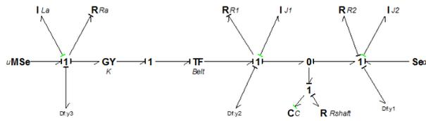
Fig. 4. BG model with derivative causality assignment
