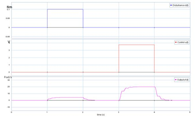
Fig. 5. Output variable  $y_1(t)$  and control  $u(t)$  without disturbance rejection
