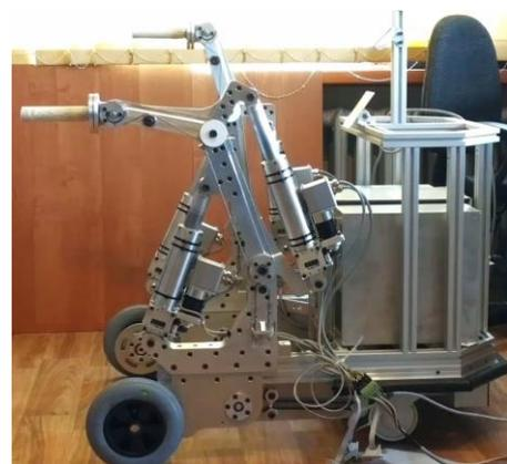
Figure 1: The MOBOT assistance robot
