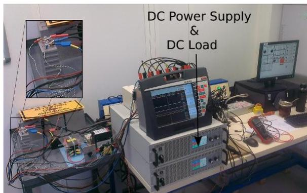
Figure 4: Battery Test Bench developed in the LAPLACE.
