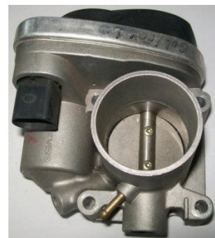
Figure 2: Volkswagen EA-111 throttle valve (Author).
