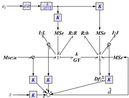
Fig. 3. Observer with the bond graph representation
